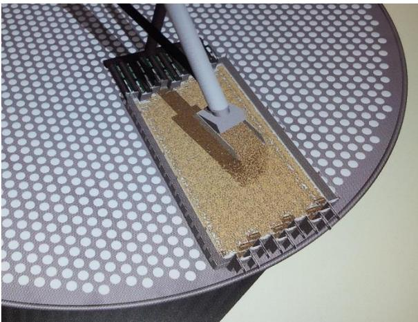
MIDC loader stands for Modular Insert De-dusting Catalyst loading system. The MIDC loading system improves on techniques already performed by Mourik, like template loading and machine loading.
