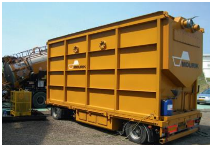
Scrubber on platform trailer for treating vacuum truck offgases
