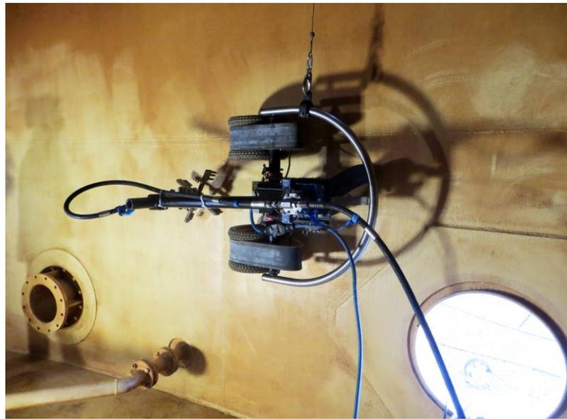
▲ A pendulum arm increases the cleaning range of the Magnetic Crawler
